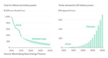
The first lithium ion cells produced by Sony Corporation in the 1990s had energy density levels of roughly 90Wh/kg and cost USD 2,000/kWh. Today's Panasonic batteries used in Tesla's Model 3 are estimated to have an energy density of 300Wh/kg and cost less than USD 200/kWh. That the total cost of the Model 3's battery pack is already two years ahead of industry forecasts made only a month before the Model 3's unveiling illustrate the rapid advances in battery technology.
